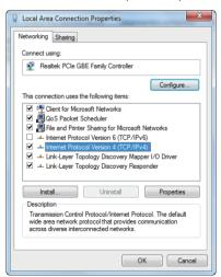
Choose Use the following IP address, input 192.168.1.200 as IP address, 255.255.255.0 as Subnet mask, and then click on OK, click on OK again.
