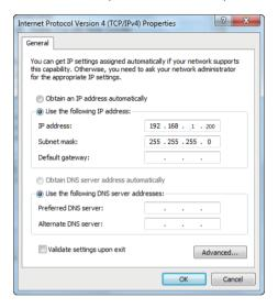
*Note:* The IP address of the computer and matrix should be in the same network segment. As the matrix's IP address is 192.168.10.100, the computer's IP should be 192.168.10.X (X contains 1~255 except 100).
