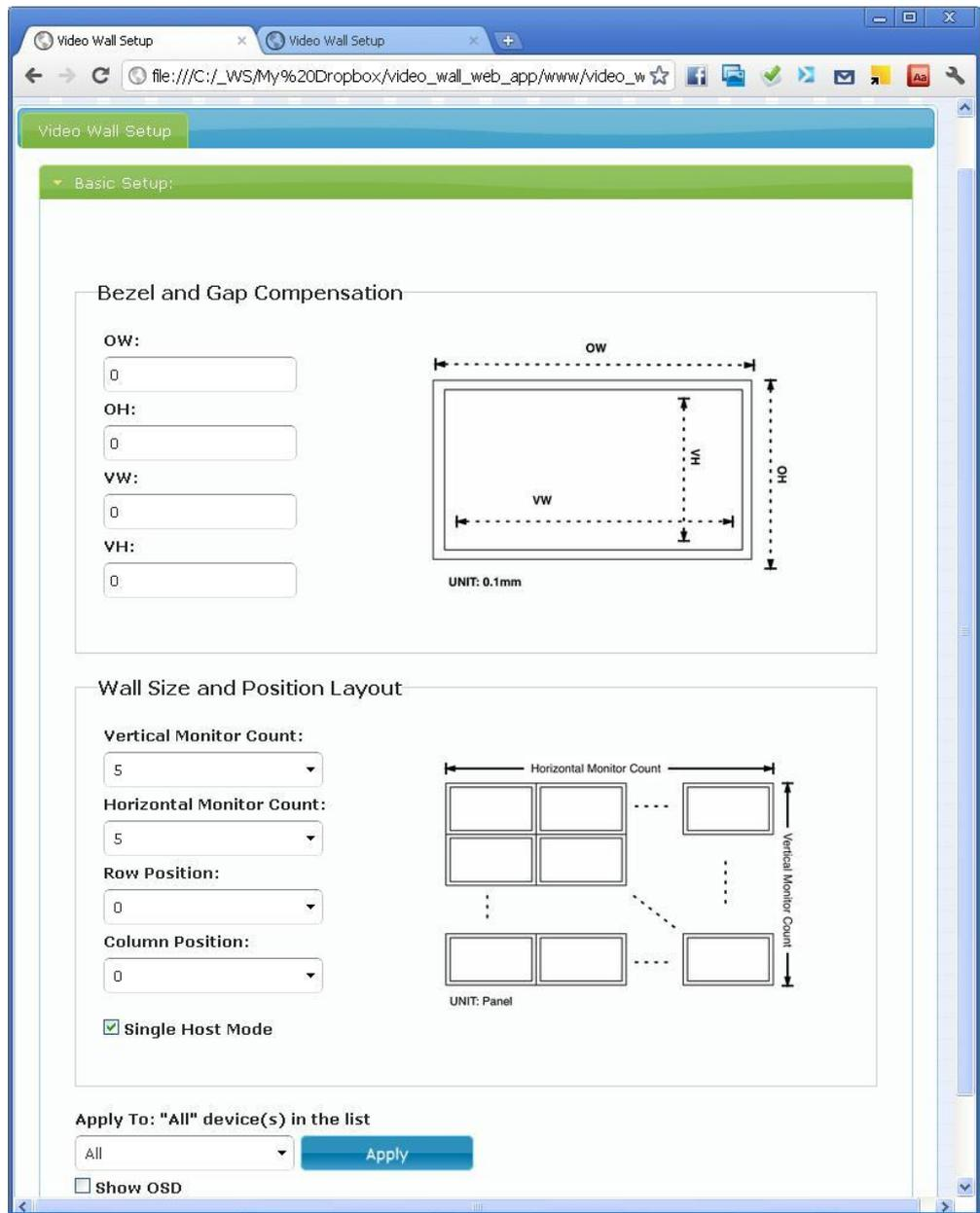
4. Once you complete the following steps in "Basic Setup", a basic video wall configuration is done.
