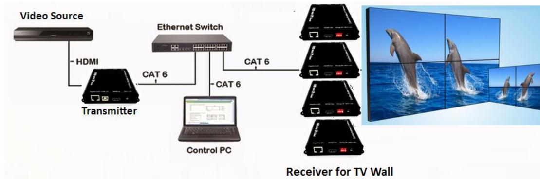
1. Connect the host (Transmitter) to the Video Source using a HDMI cable and to the Gigabit Ethernet Switch with a CAT6 cable.
