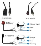
Note: When the angle between the IR receiver and the remote control is  $\pm$  45 °, the transmission distance is 0-5 meters; when the angle between the IR receiver and the remote control is  $\pm$  90 °, the transmission distance is 0-8 meters.
