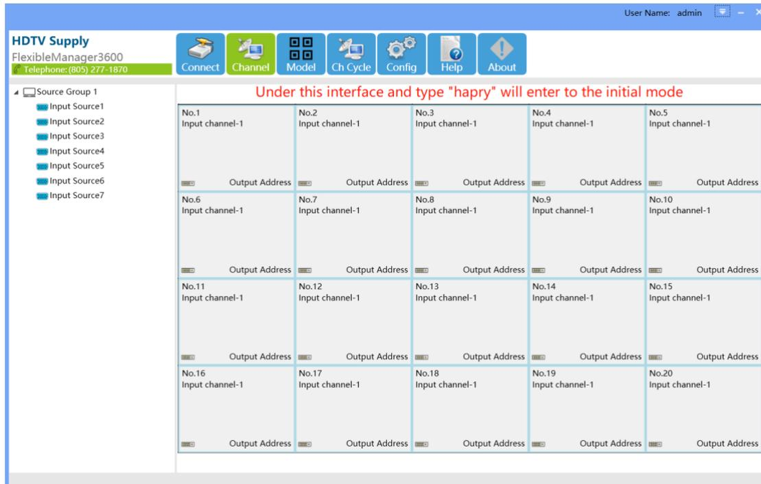
3. Click “Config” and go to “Output”, will see the “Init” button besides the “Setting”, then click “Init” to initialize the configuration. Will need to restart the matrix switcher after initialization.
