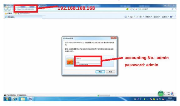
5. Enter into this new interface, control the switch by Web interface (only RJ45 port 23 or RJ45 port 24 can do that).
