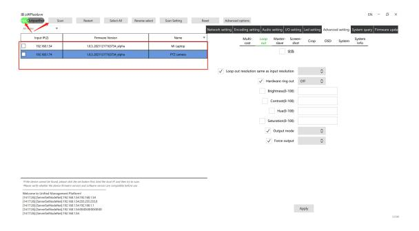
**Step 3**: Click the Output, and then "Scan" to do any settings for all the output nodes. After done the settings, the software will show a pop-up window for the operation status or showing to restart the devices which just set.
