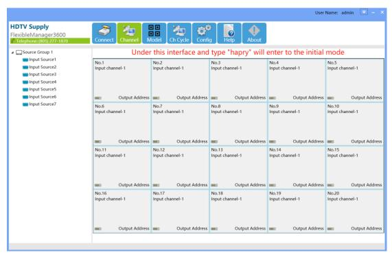
3. Click "Config" and go to "Output", will see the "Init" button besides the "Setting", then click "Init" to initialize the configuration. Will need to restart the matrix switcher after initialization.
